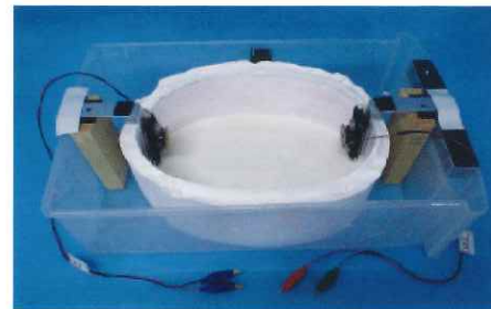
Fig. 2 Small-size water tank Water tank for the measurement of sound distribution in plaster-made phantom skull Phantom Size: 210 x 160 x 60 cm (W x D x H), Thickness: 2 cm
