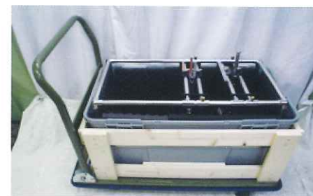
Fig. 4 Middle-size water tank Water tank for measurement of ultrasound intensity and sound distribution in skull model. Size: 70 x 40 x 35 cm (W x D x H)
