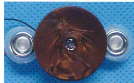
Fig. 1 Ultrasound vibrator 30 kHz frequency, vibrating surface with a 28-mm diameter, and 2 holding buttons
